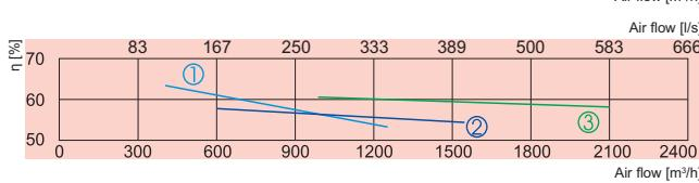
Calculated temperature efficiency (balanced mass flow) EN 13141-7:
