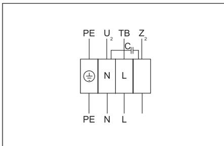
**Wiring diagram No. 1 (1~230V)**
